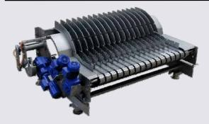
Bottle insert with one-finger-system on a crank drive. By swivelling mounting of the fingers a wear resistant one-finger-disconnection is attained.
