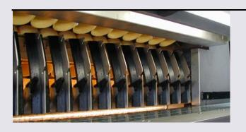
Bottle output with one-finger-system. The bottles are discharged from the cells without any fall! Pushing over with parallel continuos delivery table guarantees high stability.
